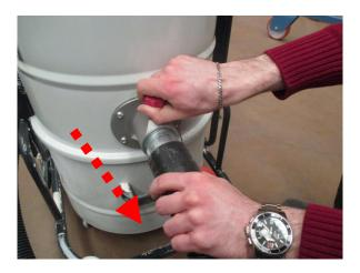
Turn on motors and then proceed to close the suction inlet with the cap attached to the suction inlet itself, assuring that there is no air flow through the filtering chamber.
